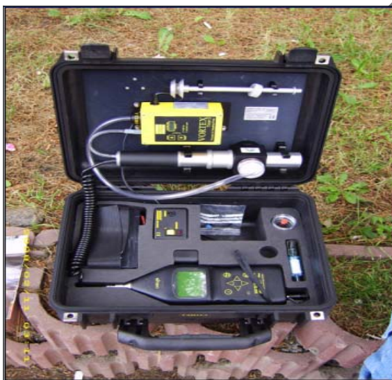
Fig. 2. MicroDust pro instrument used for PM monitoring.
