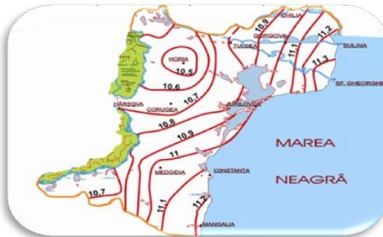
Fig. 8. The distribution of average net solar radiation (MJ / m 2 / day) during warm (APRIL-OCTOBER) in Dobrudja (1965-2005)
