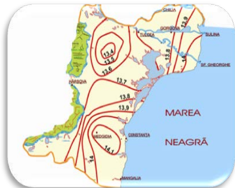
Fig. 2. The distribution of mean annual global radiation ( \text{MJ} / \text{m}^2 / \text{day} ) in Dobrudja (1965-2005)
