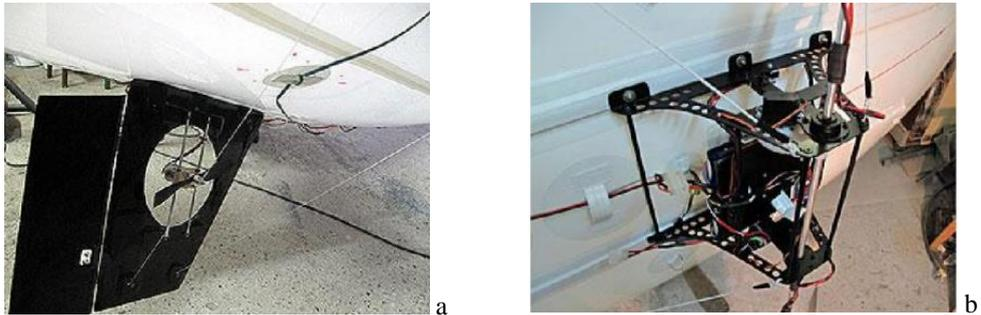
*Fig. 3. The hull blimp, a. electric motor for yaw axis, b. radio-electronic devices*
