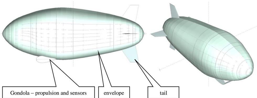
*Fig. 11. LTA geometry for analysis*
