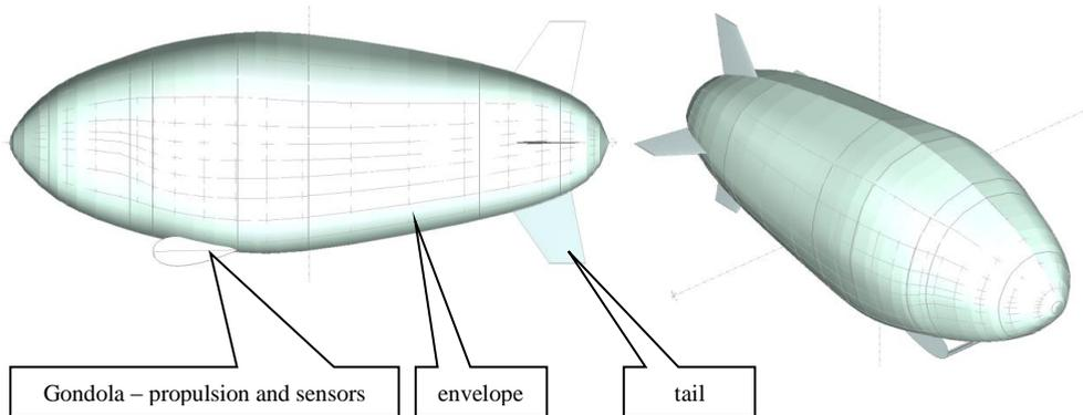
**Fig. 11. LTA geometry for analysis**
