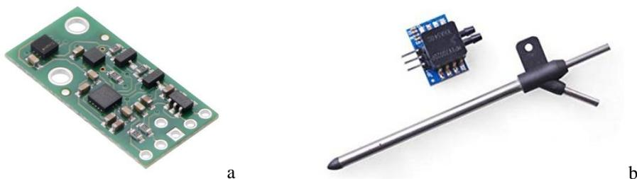
*Fig. 4. Navigation sensors - a. IMU sensor, b. Pitot sensor
