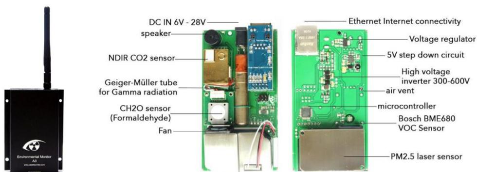
**Fig. 8. uRAD monitor model A3, (Chunhua and Kovacs, 2012).**
