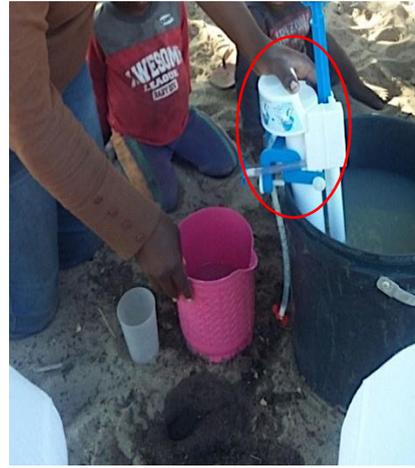
**Fig. 1. Picture of Grifaid® filter as attached to a bucket (Fig. 1a and Fig. 1b).**
